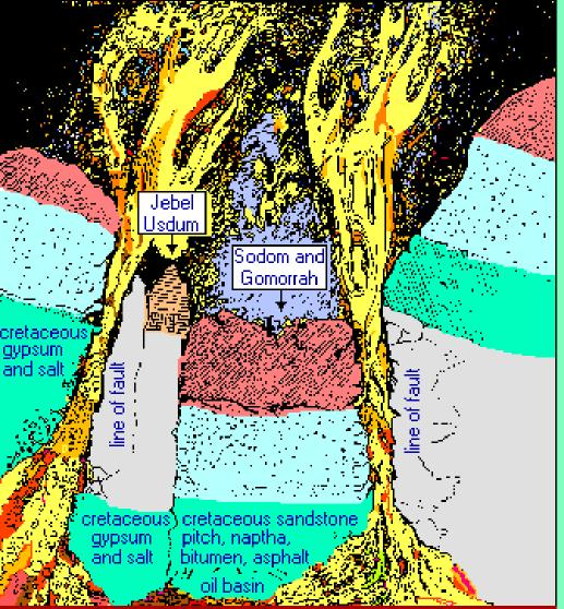
Diagram illusustrating how excessive pressure caused by faulting resulted in ignition of oil, gas, sulphur and bitumen from the underlying oil field.
